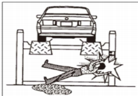
Figure 35 - Slip and fall risk
